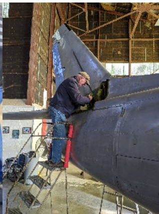
Joe Wulfkuhle fits a fairing to the F-86H
